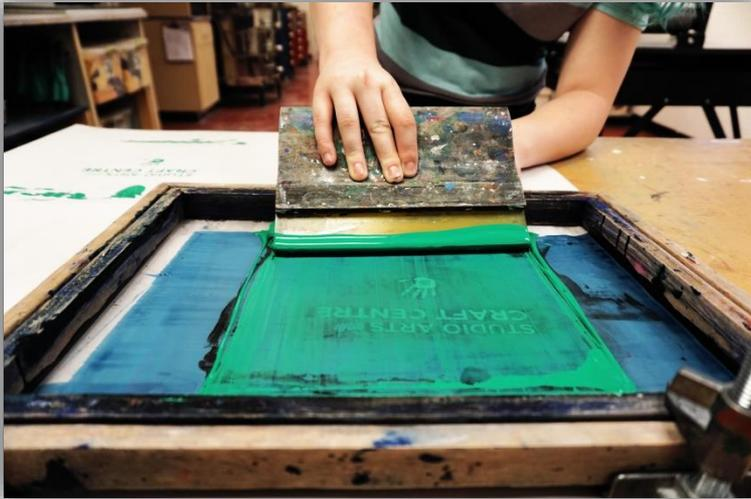
**A blade is pulled across the surface, pressing the print media through the stencil on the surface.**
